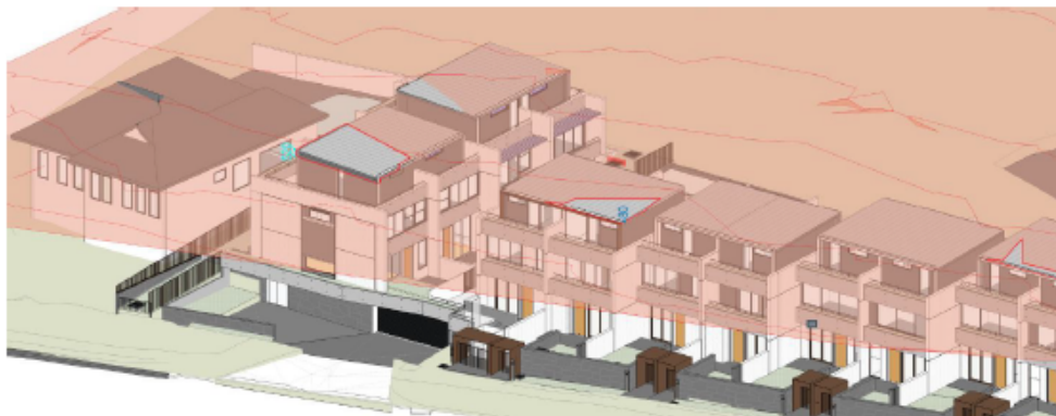
Figure 2: Extract from architectural plans noting area of roof which exceeds the 9.0m height standard (9.52m maximum height proposed) (Source – Architecture Urbaneia)
