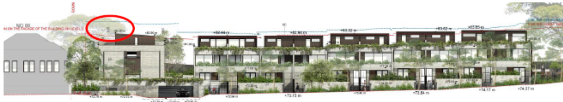
Figure 1: Extract from architectural plans noting area of roof which exceeds the 9.0m height standard (9.52m maximum height proposed) (Source – Architecture Urbaneia)
