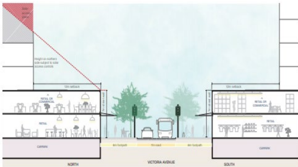
Figure 1: Section of Victoria Avenue frontage
